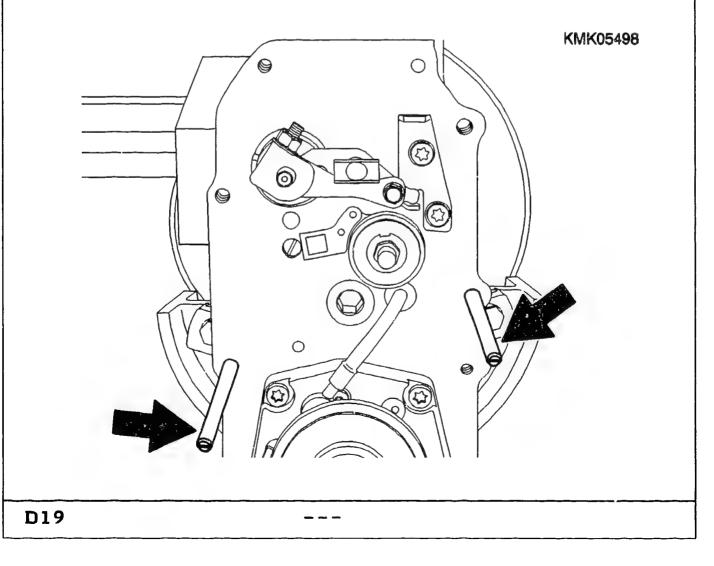
Screw out guide bolt. Screw in remaining fastening screws and tighten to torque of 7...9 Nm.
